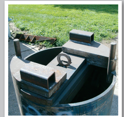
Heavy duty lock & release for the clam core doors
